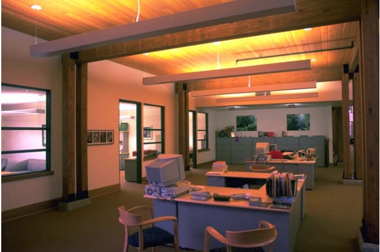
Figure 4 Minimize direct glare with indirect lighting.
